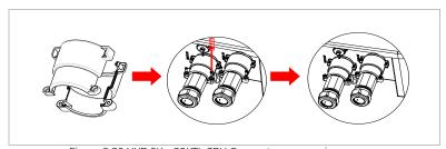
Figure 5-20 HYD 5K ... 20KTL-3PH Connector accessories
