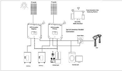
Figure 3-9 System with multiple inverter
