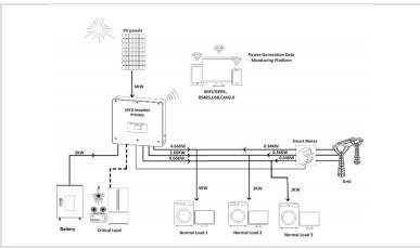
Figure 3-12 Unbalanced load (On Grid)
