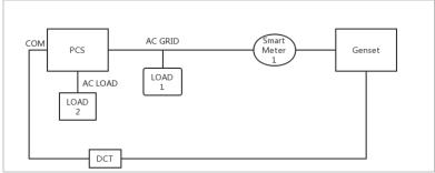
Figure 5-28 Dry Contact Wiring Diagram
