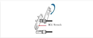
Figure 5-12 Connecting PV(d)
