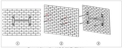
Figure 4-6 Installing HYD 5...20KTL-3PH(a)
