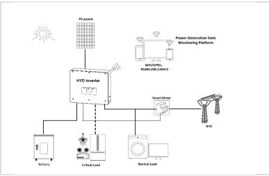
Figure 3-1 HYD 5K...20KTL-3PH inverter system diagram
