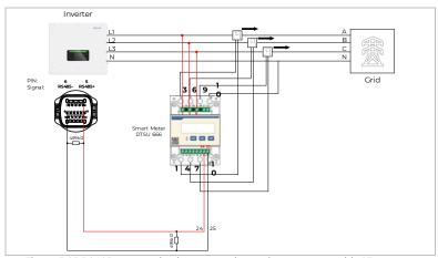
Figure 5-25 RS485 communication connection and smart meter with CTs
