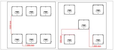
Figure 4-4 Minimum distances for several inverter
